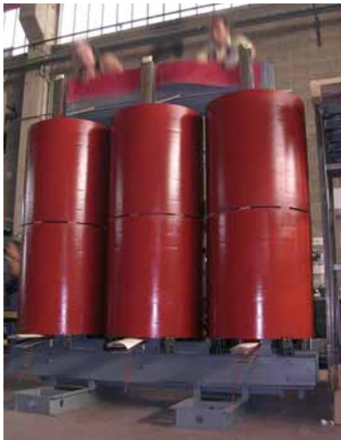
NUCLEO CON AVVOLGIMENTI BT/MT - MAGNETIC CORE WITH LV/MV WINDINGS
